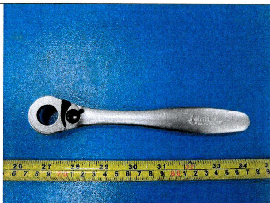
Photo "A" Appearance of sample -17H (3/8" Dr.) Insert-Snap Wrench
